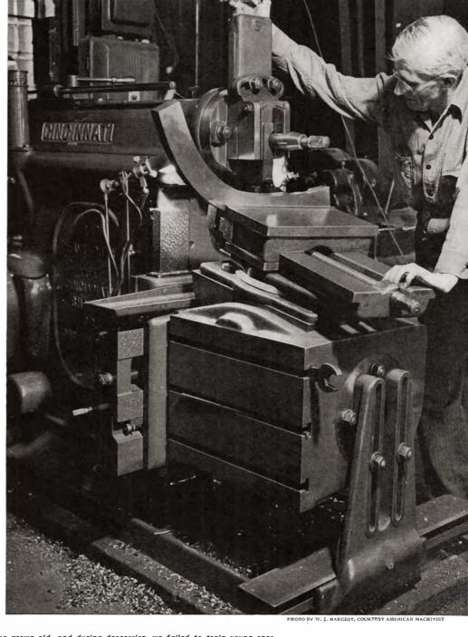
Expert machinists have grown old—and during depression we failed to train young ones. Above—Machining a die to make ribs for an airplane fuselage. Below, at left—Turning a fiver inch Navy shell in Frankford Arsenal, Philadelphia. At right—A turret lathe in operation.
